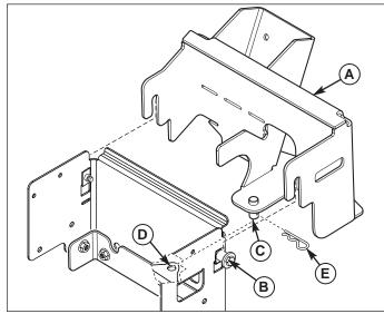
Figure 3. Hitch Installation
